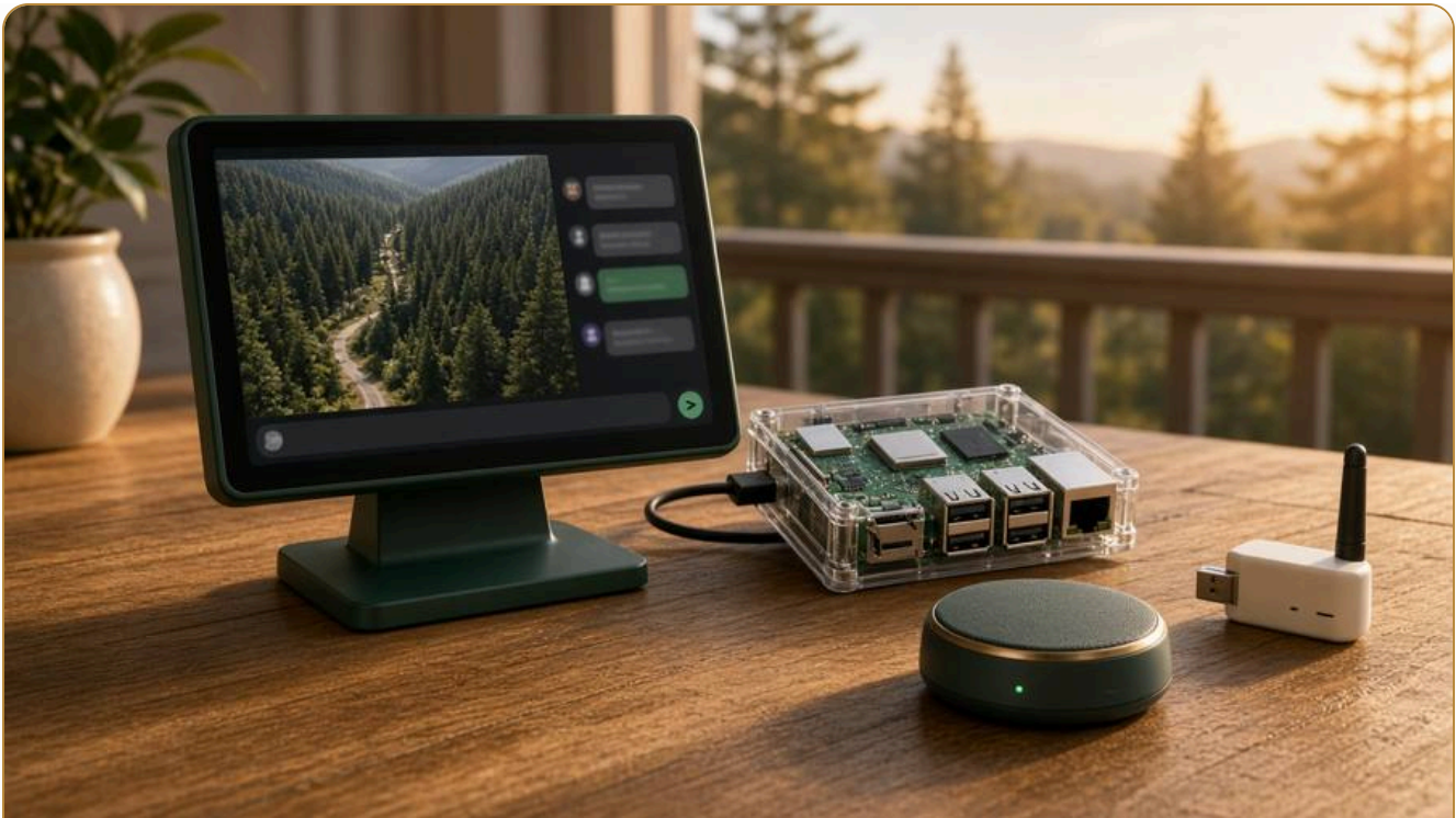
Concept render: Pi 4, 10-inch touchscreen, USB speakerphone and 5.8 GHz video receiver
