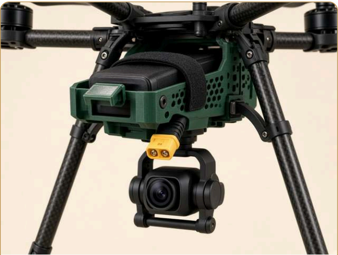
Concept render: S500 underside, showing the battery in the printed quick-swap tray with latch tab and rubberized strap, the XT60 lead, the tall carbon landing gear, and the 2-axis gimbal camera (drawn under the pack here; in the build it sits forward of the pack)
