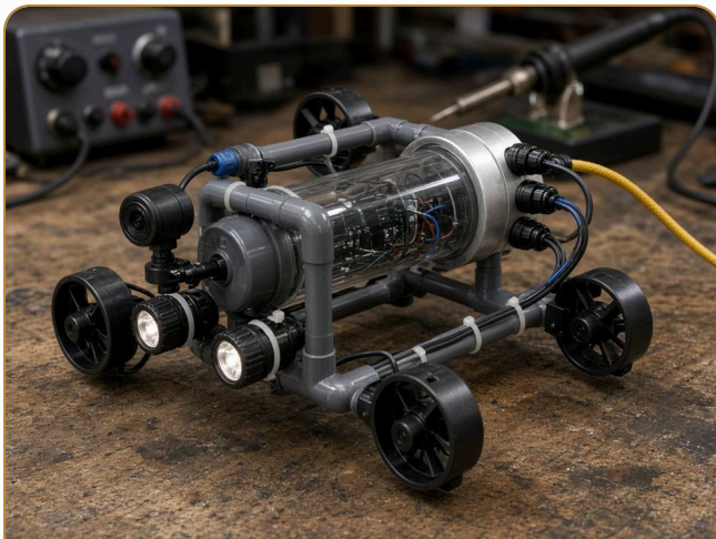
Concept render: Stage 2 with a 3-inch sealed pod, four thrusters and two dive lights
