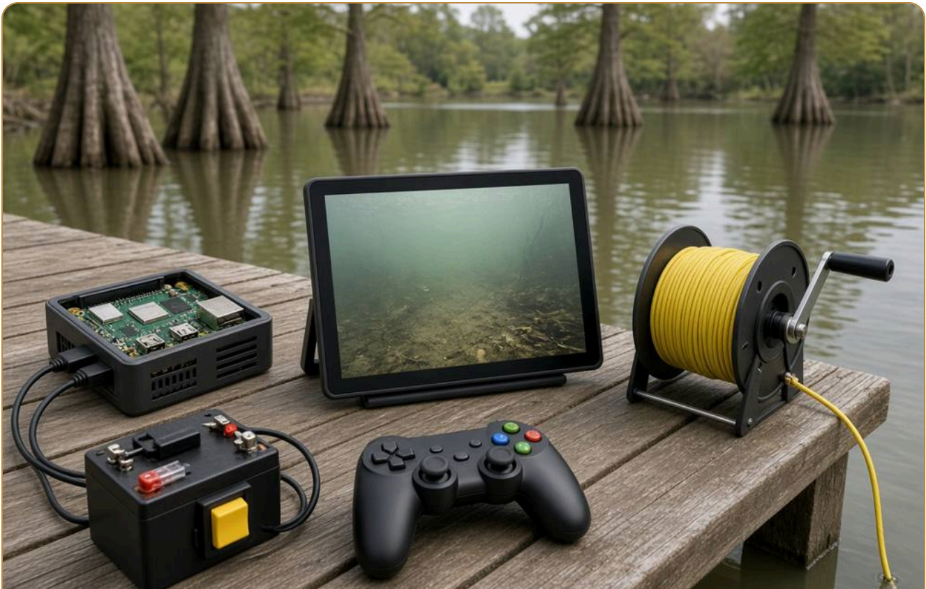
Concept render: Pi 4, 10-inch touchscreen, fused 12 V battery box, controller and tether reel on the dock
