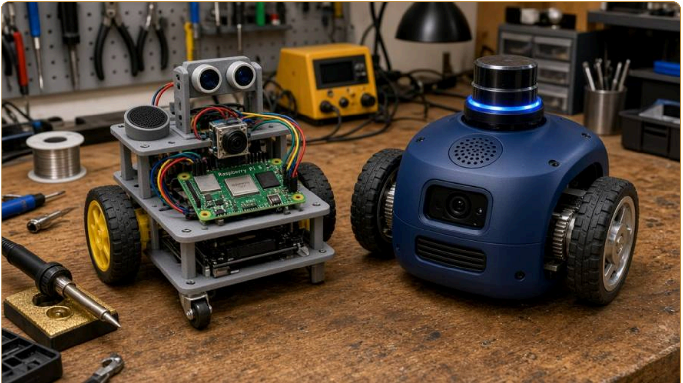
Concept render (AI-generated): left, an open-frame minimal rover with a Raspberry Pi, a camera, and ultrasonic sensors; right, an enclosed blue base with a lidar puck on top. Bases only, no torso or arms shown.
