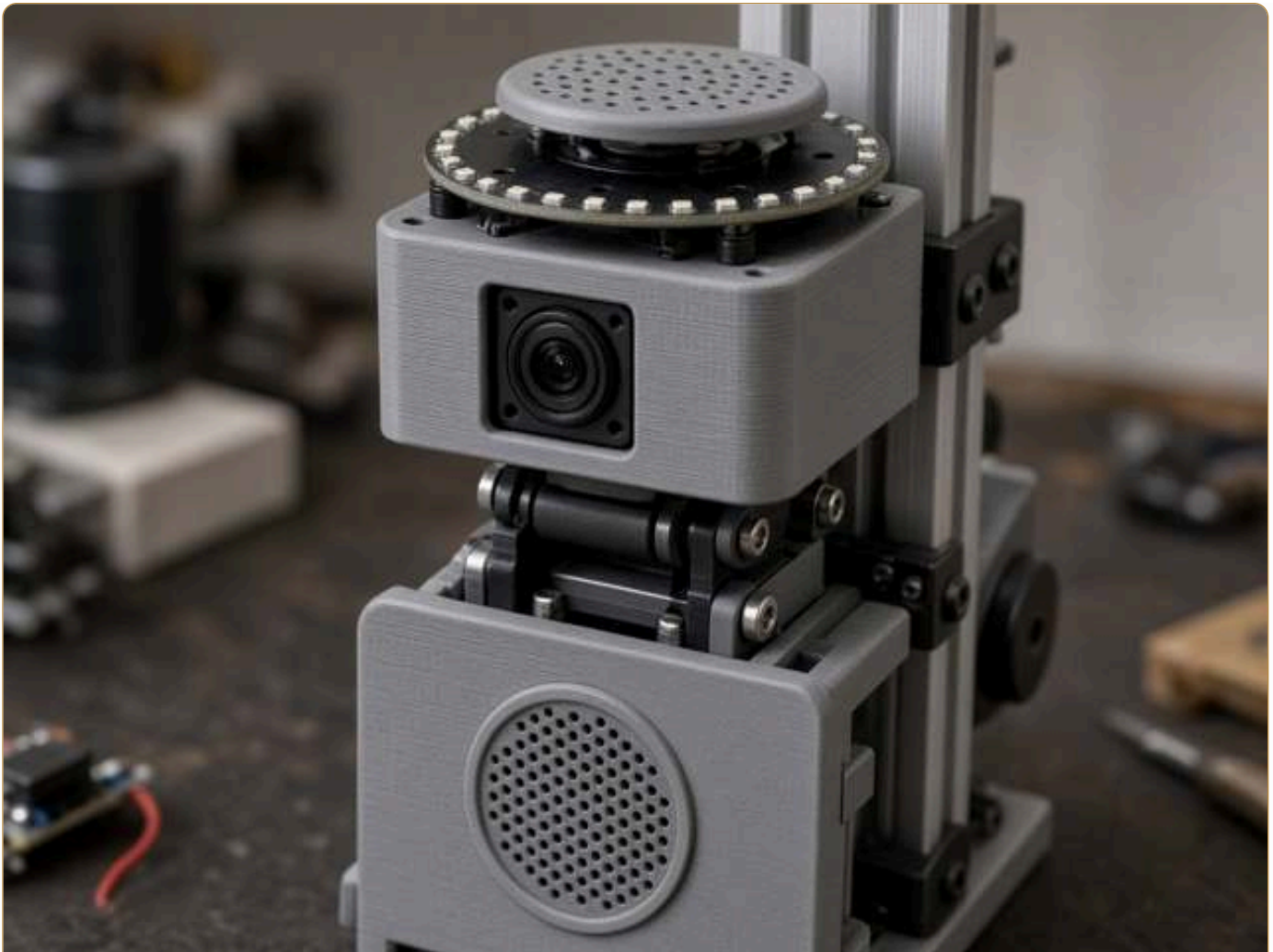
Concept render (AI-generated): head and chest close-up. The round 4-mic array sits flat on top of the head, away from the motors; the speaker grille is on the chest panel below, so the mics are not right next to the speaker.
